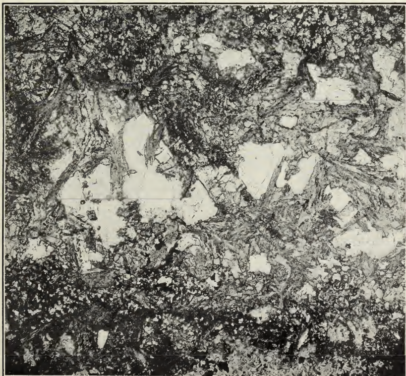
B. THIN SECTION OF WALL ROCK ADJOINING QUARTZ-WOLFRAMITE VEIN. Magnification 32 diameters. Showing an intergrowth of hornblende, vesuvianite, and fluorite.
